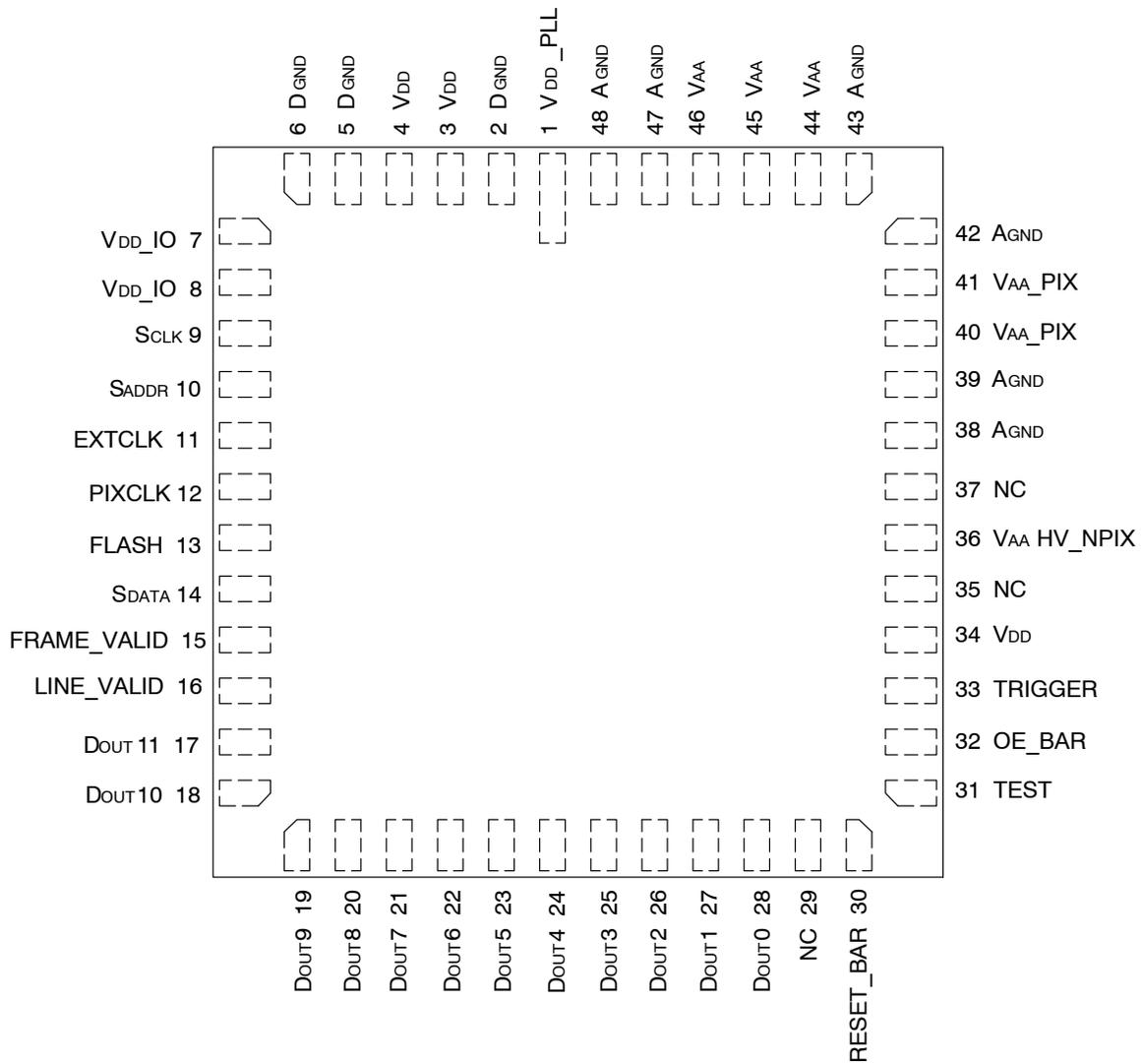
**Figure 4. PLCC Pinout**
