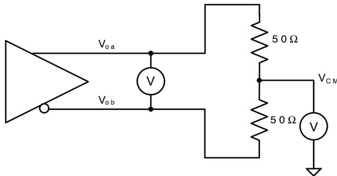
**Figure 10. DC Test Circuit**
