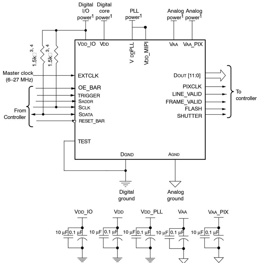
12. All power supplies must be adequately decoupled. ON Semiconductor recommends having 10 µF and 0.1 µF decoupling capacitors for every power supply. If space is a concern, then priority must be given in the following order: VAA, VAA\_PIX, VDD\_PLL, VDD\_IO, and VDD. Actual values and results may vary depending on layout and design considerations.
