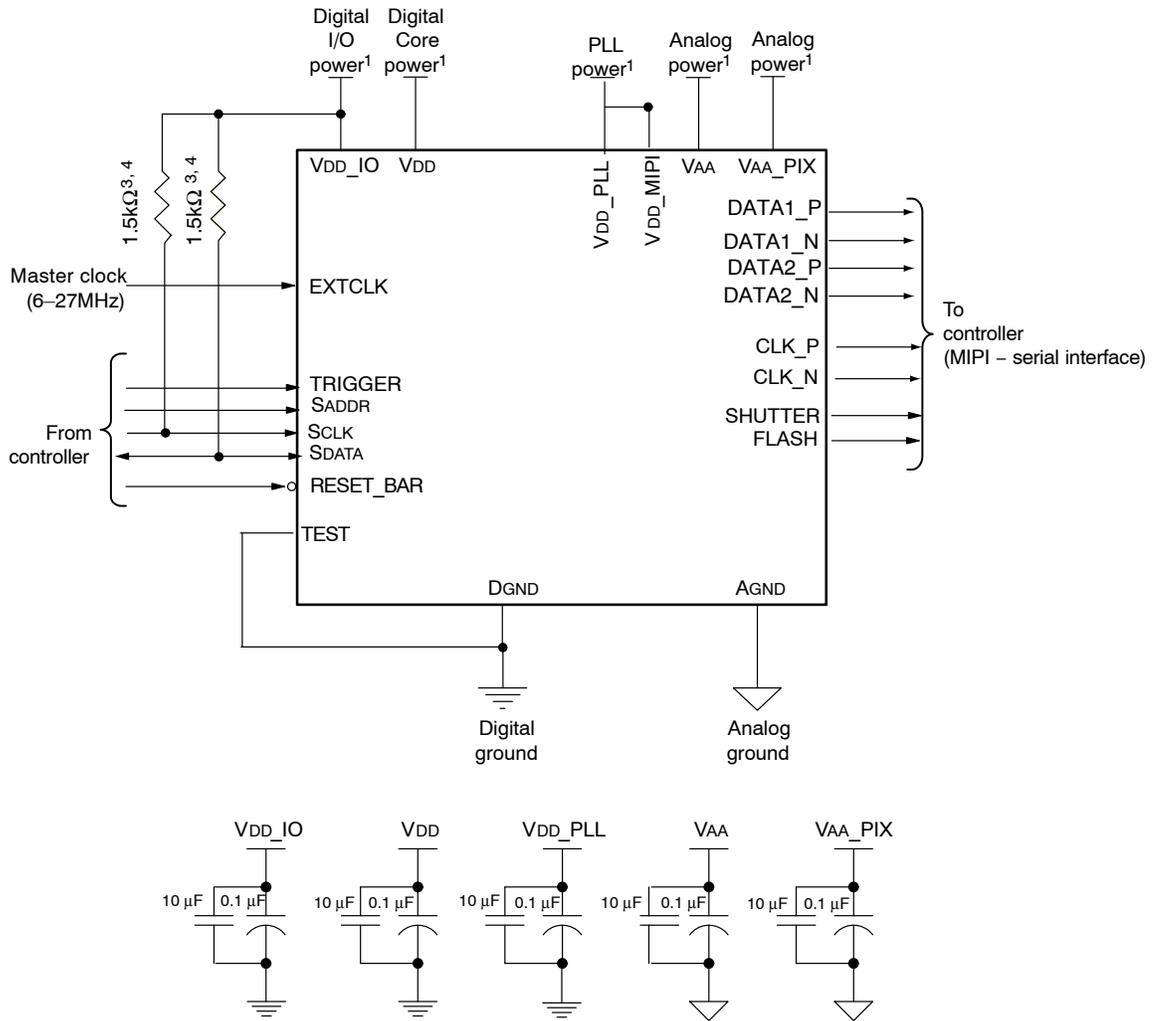
1. All power supplies must be adequately decoupled. ON Semiconductor recommends having 10 μF and 0.1 μF decoupling capacitors for every power supply. If space is a concern, then priority must be given in the following order: VAA, VAA\_PIX, VDD\_PLL, VDD\_MIPI, VDD\_IO, and VDD. Actual values and results may vary depending on layout and design considerations.
