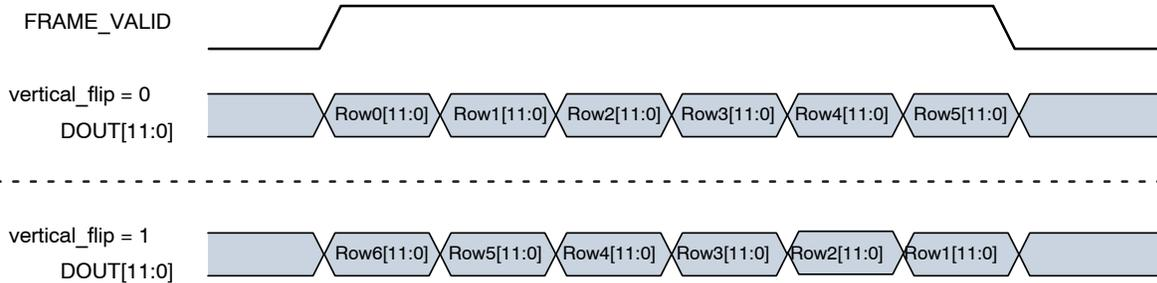
Figure 26. Effect of Vertical Flip on Readout Order
