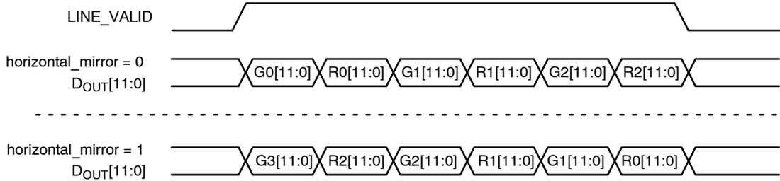
Figure 25. Effect of Horizontal Mirror on Readout Order
