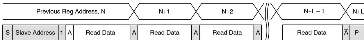
**Figure 37. Sequential READ, Start From Current Location**
