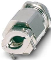
Cable gland, material for screw connection: Brass, nickel-plated, application: Standard, external cable diameter 9 mm ... 17 mm, shielding: no, connecting thread: M25 x 1.5, color: silver, with external strain relief, with O-ring
