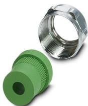
Half screw connection Pg16, made of metal, consisting of rubber seal with one hole and one pressure screw, for type 1 housings, cable [mm] 7 - 10.5
