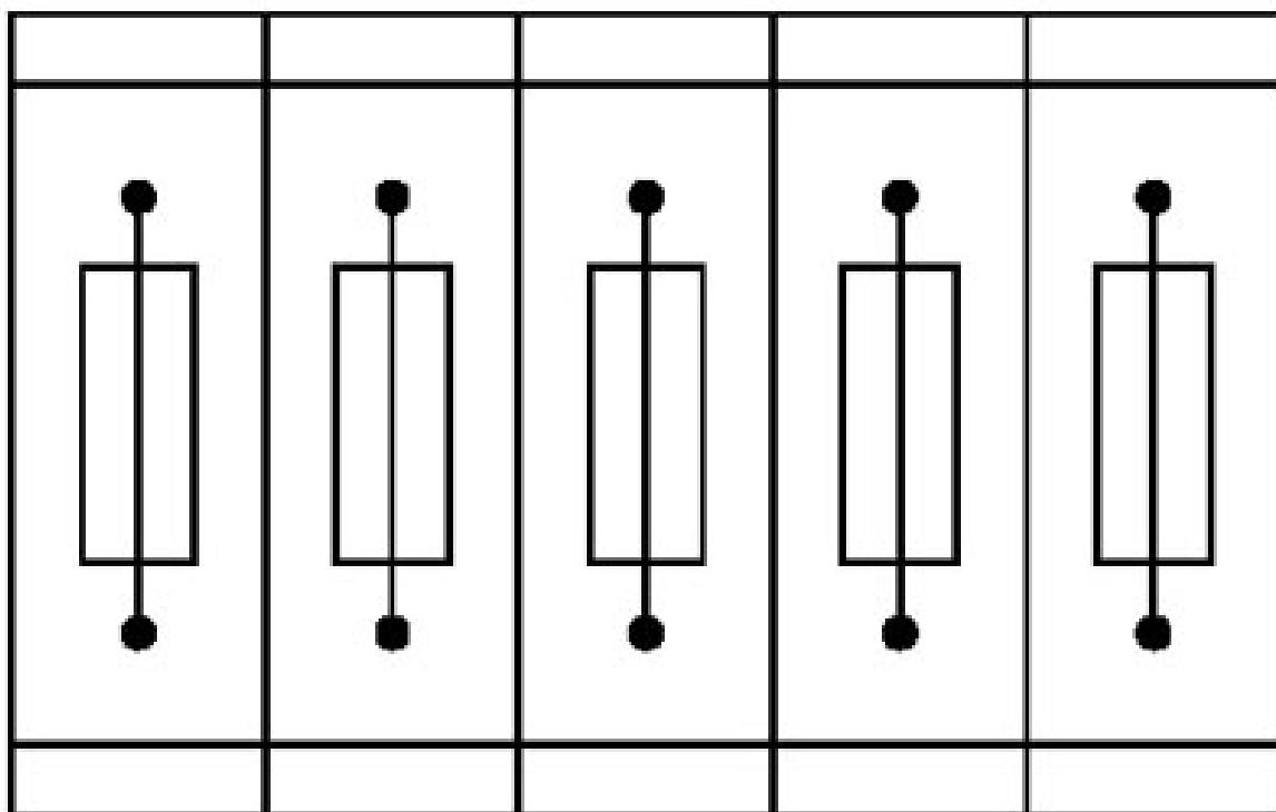
Fuse terminal blocks in interconnected arrangement,
