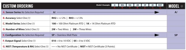
Note\*: Outputs are field selectable between 0-5 VDC & 0-10 VDC
