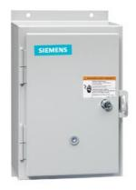
Non-reversing motor starter, Size 0, Three phase full voltage, Solid-state overload relay, OLRelay amp range 0.75-3.4a, 24VAC 50-60HZ coil, Non-combination type, Enclosure type 12, Dust/drip proof for indoors, Extra-wide enclosure
