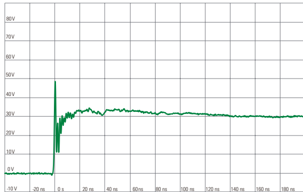
ISO10605 Contact Discharge Plot at +8 kV
