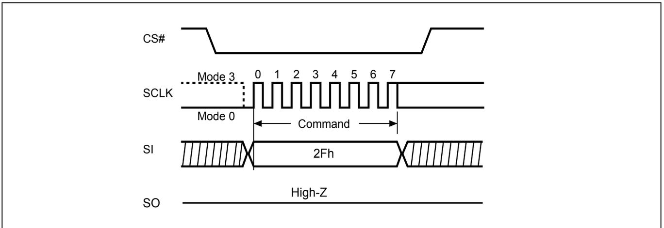
**Figure 58. Write Security Register (WRSCUR) Sequence (QPI Mode)**
