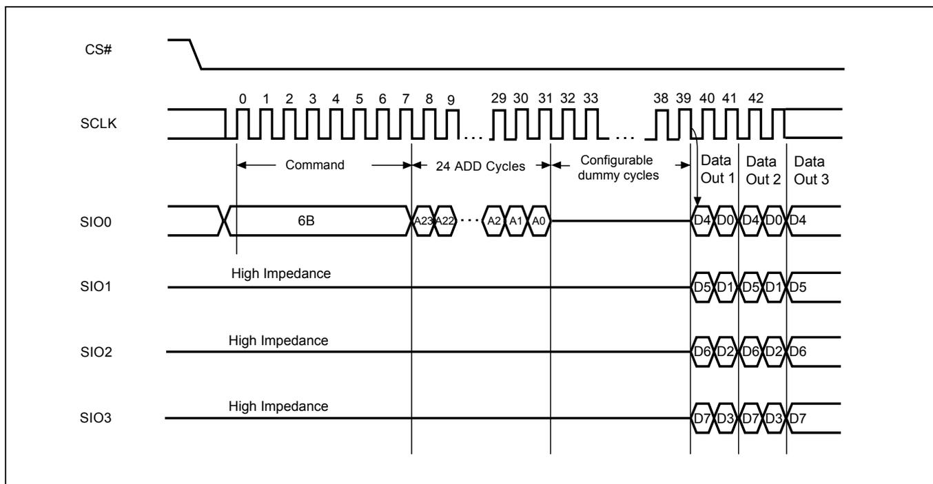
**Note:** Configuration Dummy cycle numbers will be different depending on the bit6 & bit 7 (DC0 & DC1) setting in configuration register.
