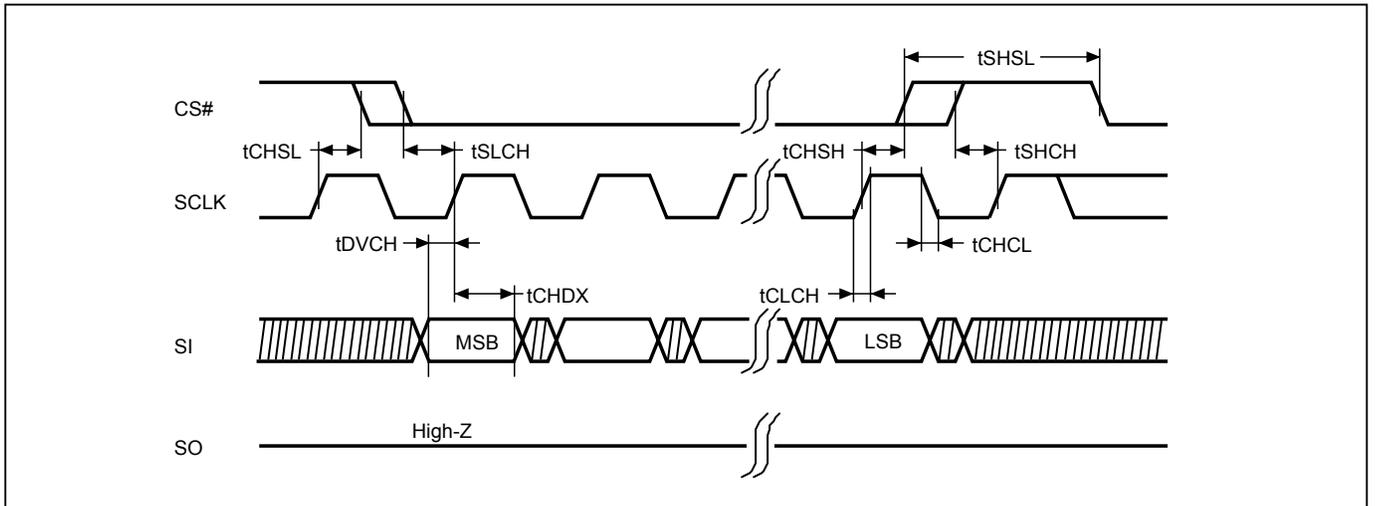
**Figure 3. Output Timing**
