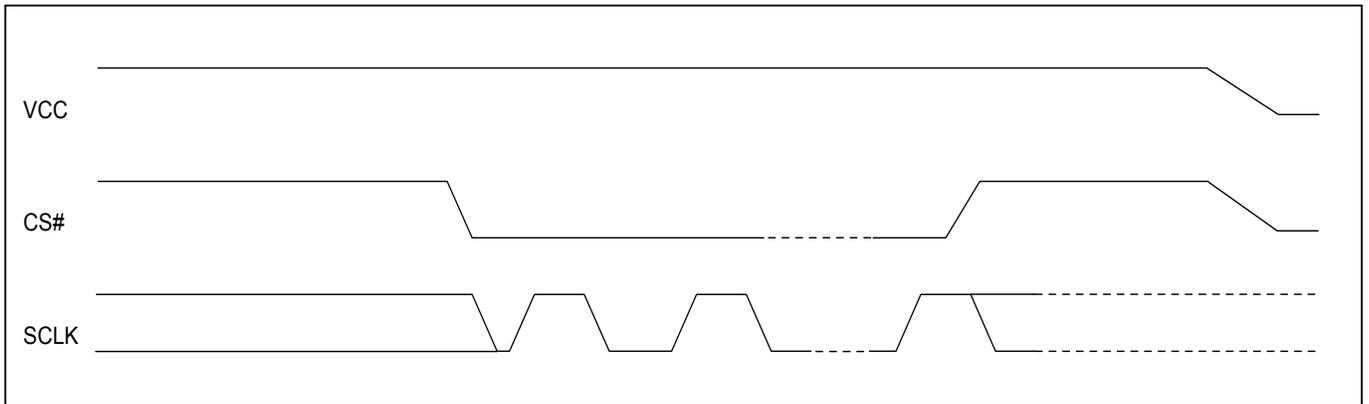
**Figure 85. Power-up Timing**
