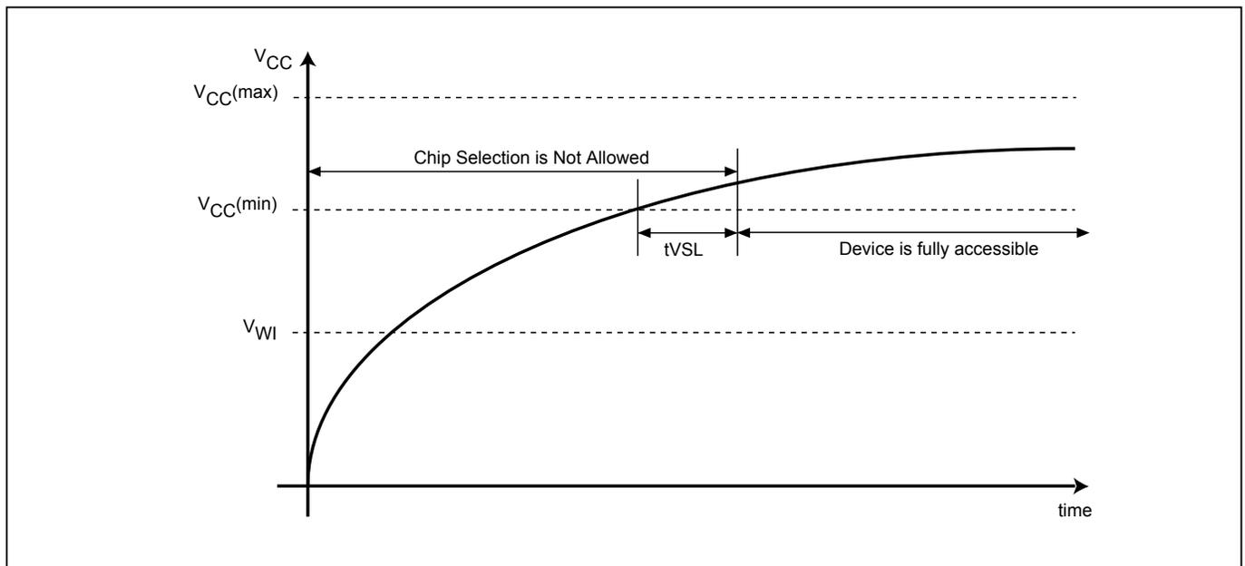
**Figure 86. Power Up/Down and Voltage Drop**
