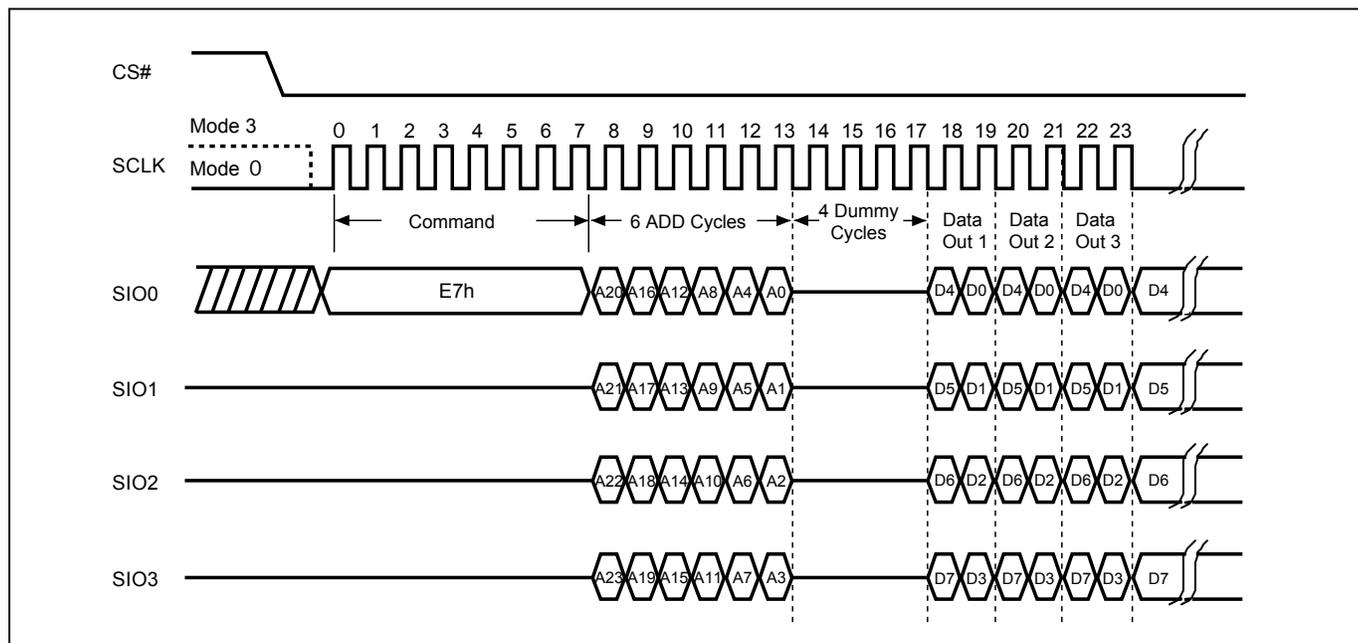
**Figure 32. 4 x I/O Read Mode Sequence (SPI Mode)**
