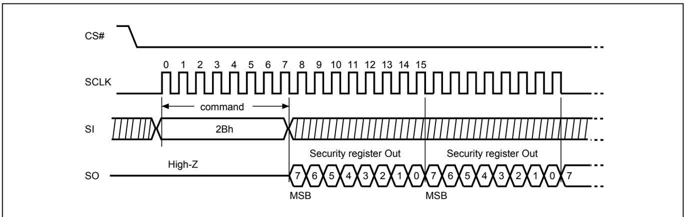
**Figure 56. Read Security Register (RDSCUR) Sequence (QPI Mode)**
