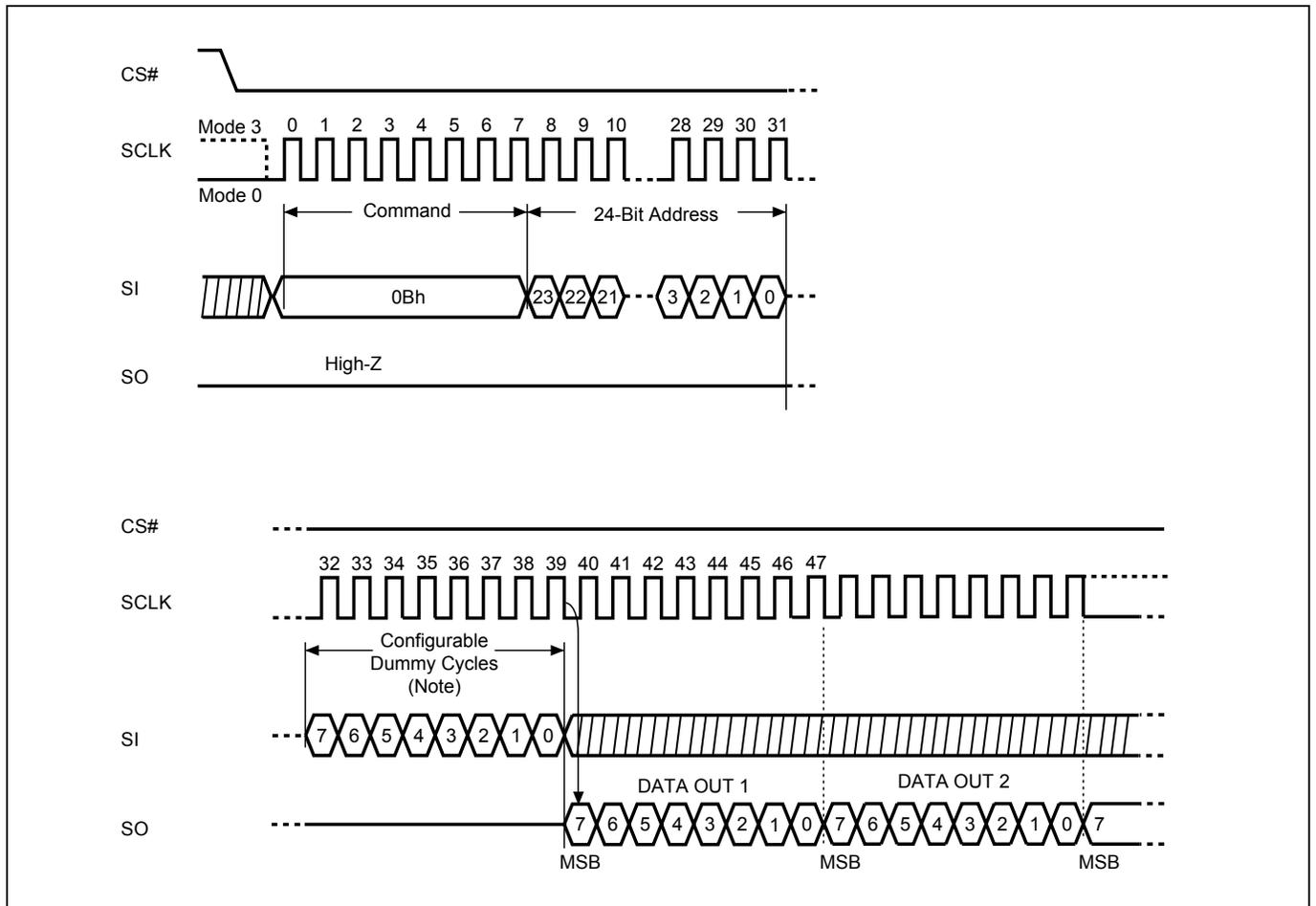
**Note:** Configuration Dummy cycle numbers will be different depending on the bit6 & bit 7 (DC0 & DC1) setting in configuration register.
