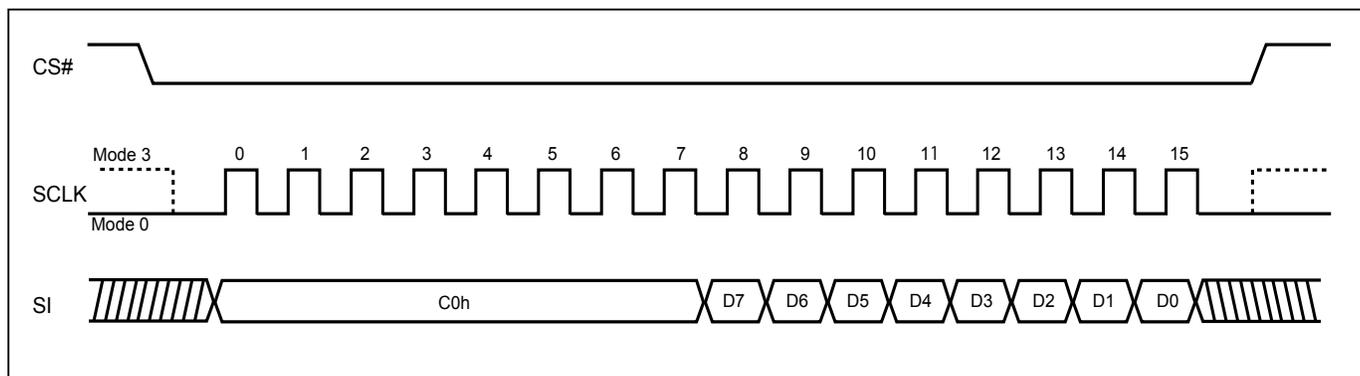
**Figure 35. Burst Read (QPI Mode)**
