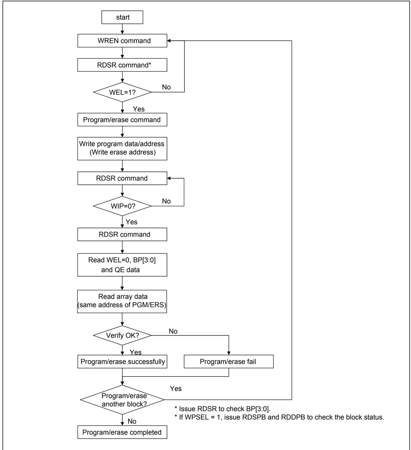
Figure 22. Program/Erase flow without read array data (read P\_FAIL/E\_FAIL flag)
