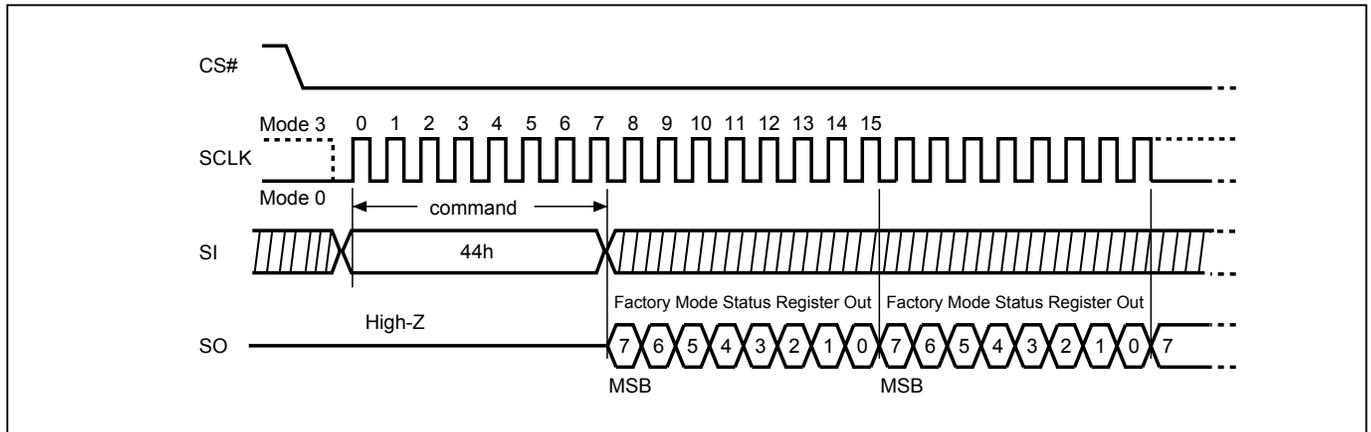
**Figure 52. Read Status Register (RDSR) Sequence (QPI Mode)**
