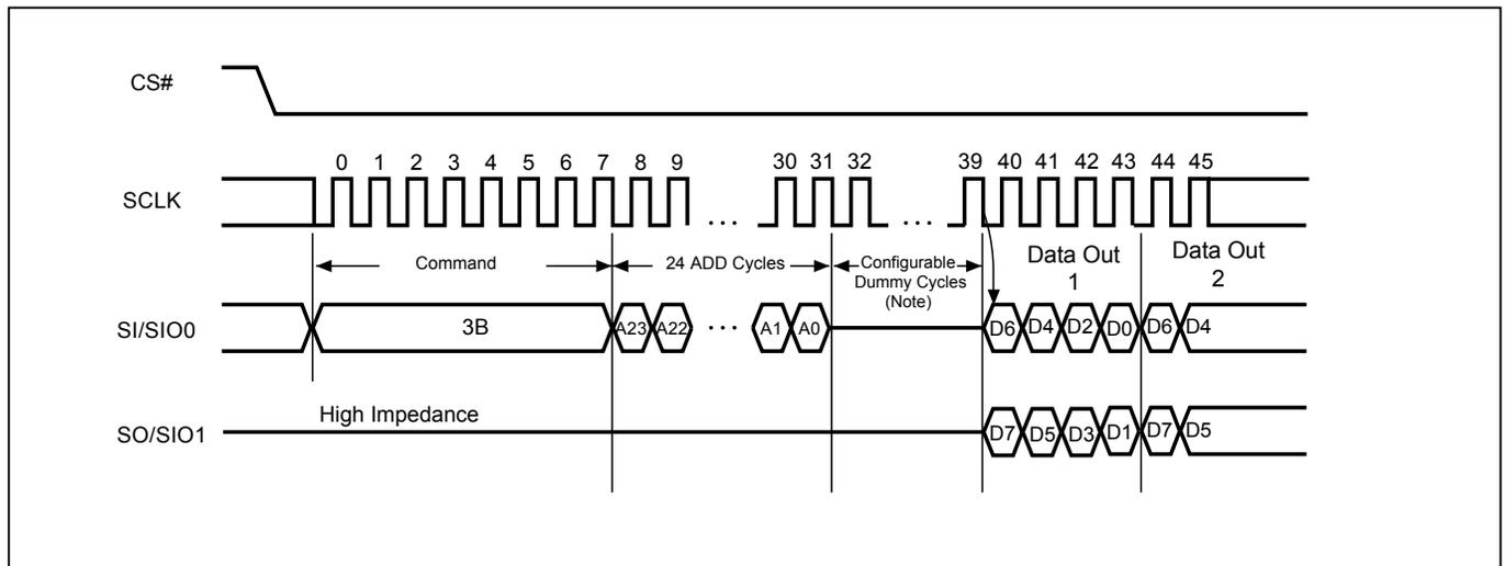
**Note:** Configuration Dummy cycle numbers will be different depending on the bit6 & bit 7 (DC0 & DC1) setting in configuration register.
