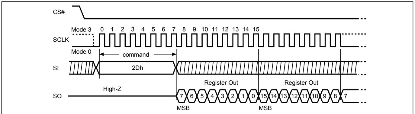
**Figure 63. Write Lock Register (WRLR) Sequence (SPI Mode only)**
