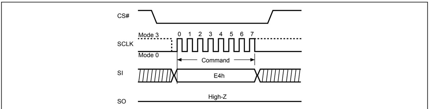
**Figure 66. SPB Program (WRSPB) Sequence (SPI Mode only)**
