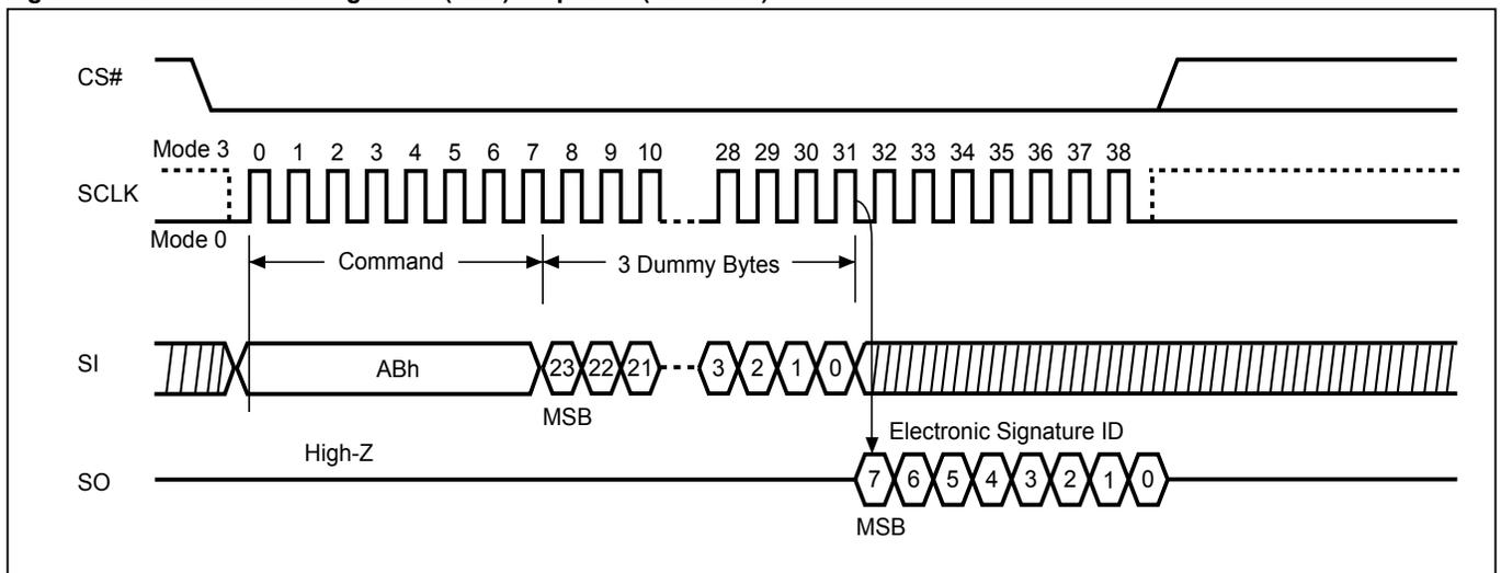
**Figure 14. Read Electronic Signature (RES) Sequence (QPI Mode)**
