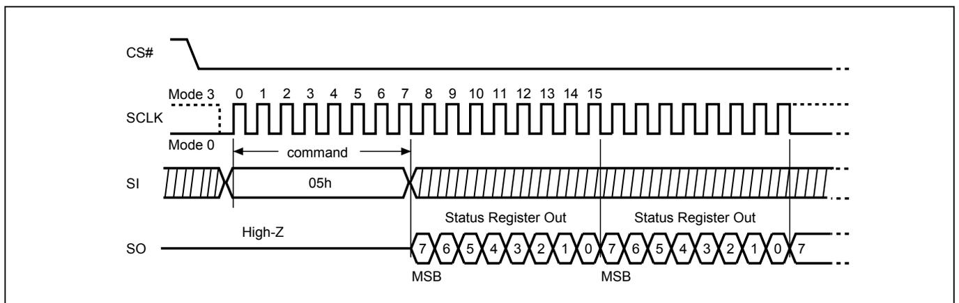
**Figure 18. Read Status Register (RDSR) Sequence (QPI Mode)**
