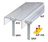
Flat-ribbon cover, for covering terminal strips, 2 mm thick, 10 cm wide, an additional requirement are 2 E/UK end brackets and 2 adjustable VAH cover holders. The max. supply length is 100 cm
