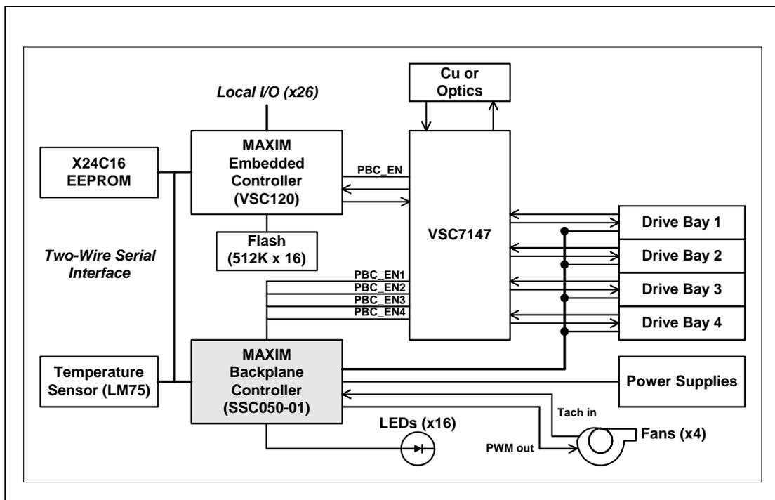
Figure 1-2. Single Loop, Single Controller with Four Drives
