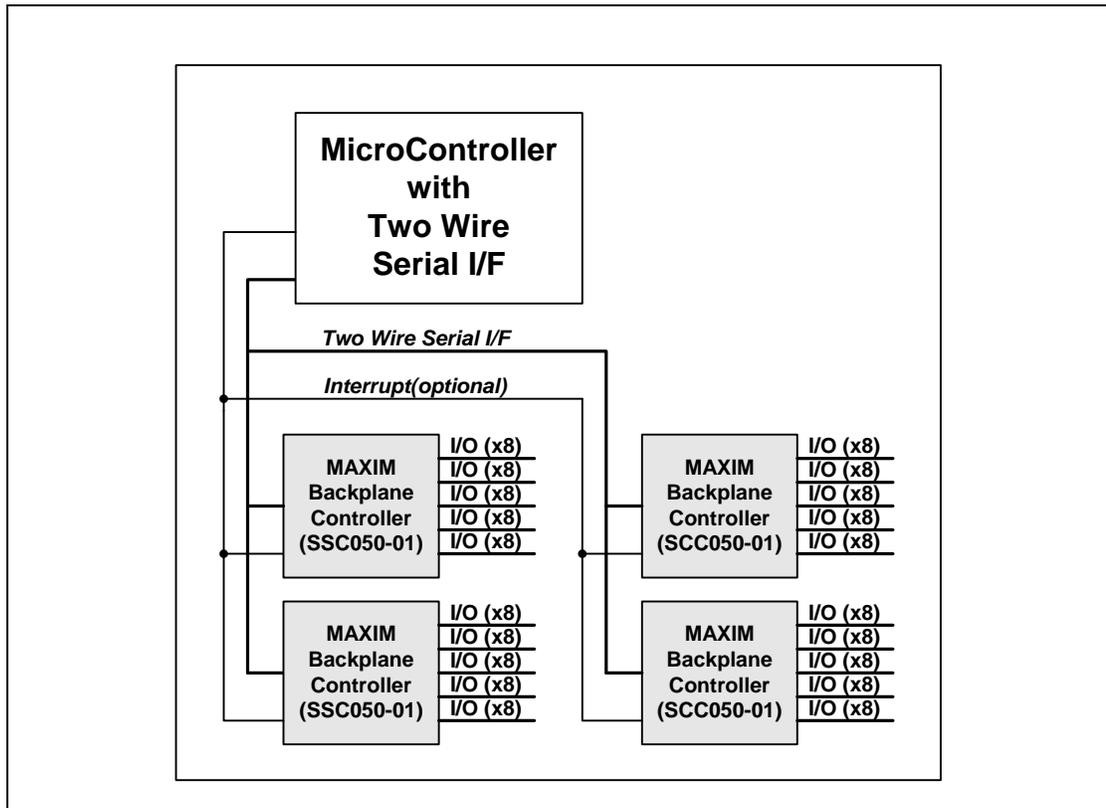
Figure 1-3. Four Backplane Controllers, 160 Bidirectional I/O Lines
