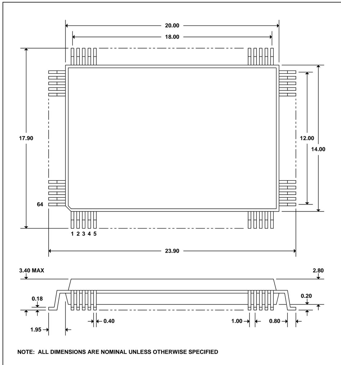
Figure 6-1. Mechanical Drawing
