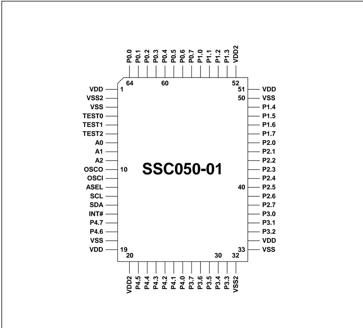
Figure 3-2. Pinout Diagram
