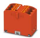
Distribution block, Basic terminal block, nom. voltage: 450 V, nominal current: 24 A, number of connections: 6, connection method: Push-in connection, cross section: 0.14  $\text{mm}^2$  - 4  $\text{mm}^2$ , mounting type: adhesive, color: red
