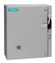
Non-reversing motor starter, Size 2 1/2, Three phase full voltage, Solid-state overload relay, OLRelay amp range 25-100A, 24VAC 50-60HZ coil, Combination type, 100A non-fusible disconnect, Enclosure NEMA type 1, Indoor general purpose use, Standard width enclosure
