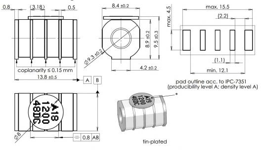
\* - for pick and place, dimension of suction nozzle should be smaller than disc
