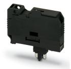
Fuse plug, Prior to replacing the cartridge fuse, disconnect the fuse connector from the basic terminal block., nominal current: 10 A, fuse type:  $G / 6.3 \times 32$ , color: black
