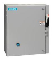
Non-reversing motor starter Size 2 1/2 Three phase full voltage Solid-state overload relay OLRelay amp range 25-100A 240V 50HZ / 277V 60HZ coil Combination type 100A circuit breaker Enclosure NEMA type 1 Indoor general purpose use Standard width enclosure
