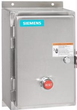
Non-reversing motor starter Size 0 Single phase full voltage Solid-state overload relay OLRelay amp range 0.75-3.4A 190-220/220-240V 50/60HZ coil Combination type Water/dust tight non-corrosive
