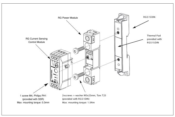
The RG Power Module is gradually tightened (alternating between the 2 screws) to a maximum torque of 1.5Nm.
