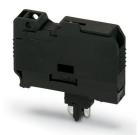
Fuse plug, Prior to replacing the cartridge fuse, disconnect the fuse connector from the basic terminal block., nom. voltage: 630 V, nominal current: 10 A, connection method: Plug-in connection, fuse type:  $G / 6.3 \times 32$ , mounting type: Plug-in mounting, color: black
