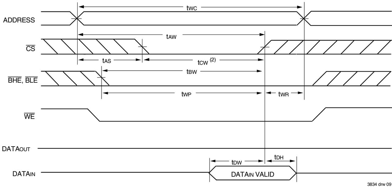
Timing Waveform of Write Cycle No. 3 ( $\overline{\text{BHE}}$ ,  $\overline{\text{BLE}}$  Controlled Timing)<sup>(1,4)</sup>
