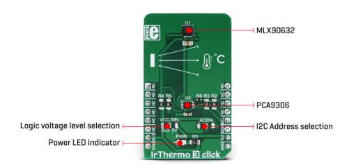
The MLX90632 FIR sensor is factory calibrated in wide temperature range: -20°C to 80°C for ambient (sensor) temperature and --20°C to 200°C for the object temperature. An integrated thermal sensor allows ambient temperature measurement independently of the thermopile itself, allowing accurate calibration calculations to be performed.
