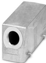
Sleeve housing B24, for double locking latch, material: Die-cast aluminum, salt water resistant, cable outlets: 1, lateral, 1x M32, height: 60 mm, cable gland: none, Standard
