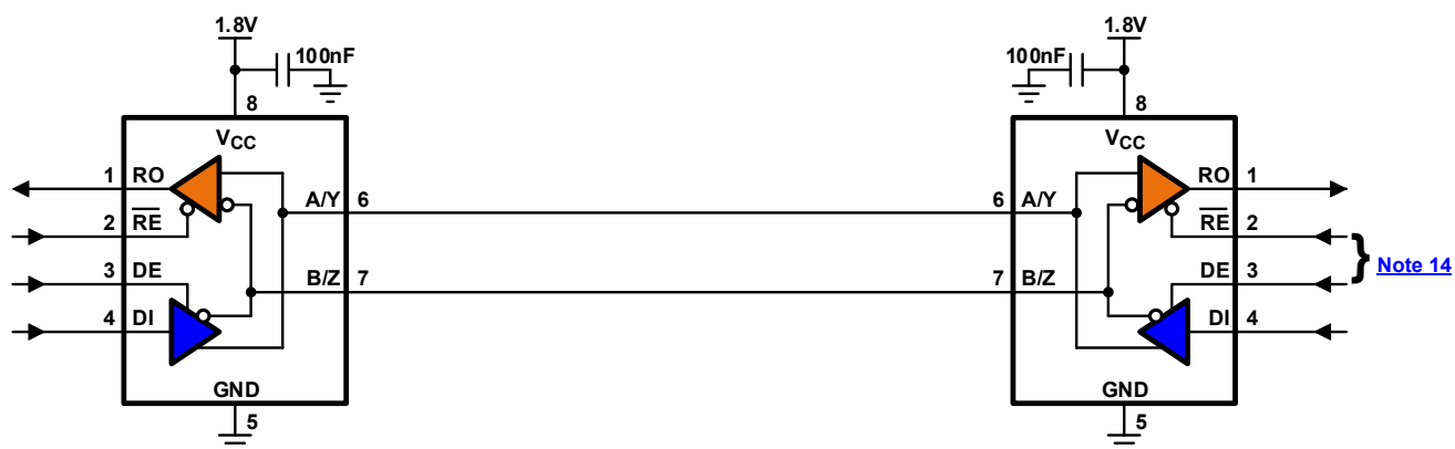
FIGURE 3. HALF DUPLEX NETWORK USING ISL32603E
