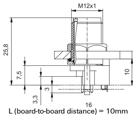
**Front panel section****PCB design**
