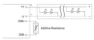
"DO NOT connect "DIM- to -V"
