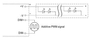
"DO NOT connect "DIM- to -V"
