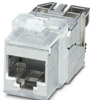
RJ45 jack insert, design: RJ45, degree of protection: IP20, number of positions: 8, 10 Gbps, CAT6<sub>A</sub>, material: Metal, connection method: IDC connection, connection cross section: AWG 26-22, cable outlet: straight, Keystone design for use with IP20 panel mounting frame or integrated directly into the housing panel, Ethernet
