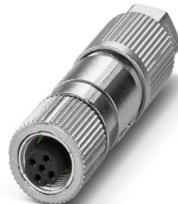
Data connector, PROFIBUS (31.25 kbps), 2-position, halogen-free, shielded, Socket straight M12, coding: A, Insulation displacement connection, knurl material: Zinc die-cast, nickel-plated, external cable diameter 5 mm ... 9.7 mm
