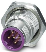
Device connector rear mounting, 5-position, Pin, straight, M12-SPEEDCON, coding: B, Rear mounting, Pg9, Solder pins, Alternative product in accordance with RoHS II without Exemption 6c (Pb < 0.1 %) item no.: 1239812
