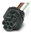
Device connector rear mounting, Range of articles: PRC 35, housing material: PPE, color: black, number of positions: 5, max. conductor cross section: 2.5 mm², rated voltage: 690 V AC, rated current: 24 A, Connection method: Crimp connection, Contact connection type: Pin, cable length: 150, This item is also available with other cable lengths. For your specific requirements, please contact your local PHOENIX CONTACT subsidiary.
