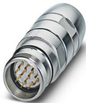
M23, Coupler connector, series: UC, straight, shielded: yes, Screw locking mechanism, No. of pos.: 16+3, Direction of rotation: Standard, contact connection type: Pin, Solder cup, coding: N
