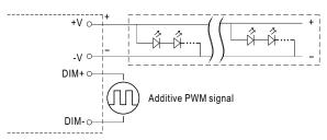
"DO NOT connect "DIM- to -V"
