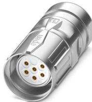
M23, Cable connector, series: CA, straight, shielded: yes, SPEEDCON, No. of pos.: 7, Direction of rotation: Standard, contact connection type: Socket, Solder connection, cable diameter range: 6 mm ... 10 mm, coding: N, Alternative product in accordance with RoHS II without Exemption 6c (Pb < 0.1 %) item no.: 1243640
