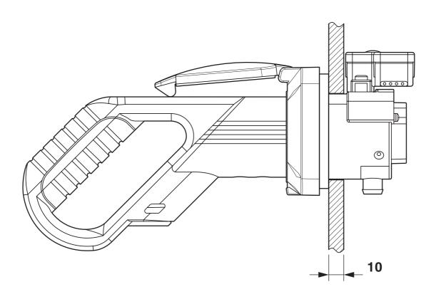
Panel thickness for front mounting (in mm)
