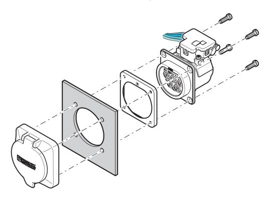
Rear mounting with rear protective cover screw connection
