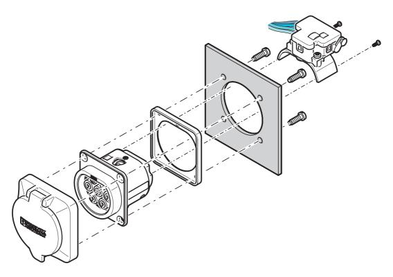
Front mounting with rear protective cover screw connection
