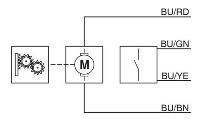
Block diagram of the locking actuator
