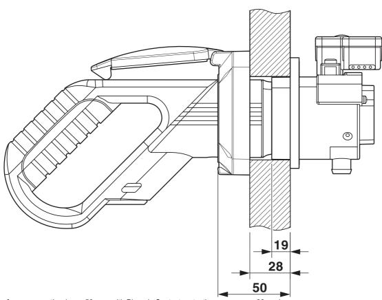
Panel thickness for rear mounting (max. 50 mm, with Phoenix Contact protective cover, max. 22 mm)
