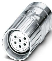
M23, Cable connector, series: CA, straight, shielded: yes, Screw locking mechanism, No. of pos.: 6, Direction of rotation: Standard, contact connection type: Socket, Solder connection, cable diameter range: 4 mm ... 6 mm, coding: N, Alternative product in accordance with RoHS II without Exemption 6c (Pb < 0.1 %) item no.: 1243802
