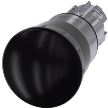
Mushroom pushbutton, 22 mm, round, metal, shiny, black, 40 mm, positive latching, acc. to EN ISO 13850, rotate-to-unlatch, with laser labeling, lower case
