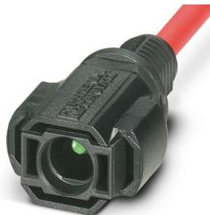
Device connector front mounting, Range of articles: SUNCLIX, housing material: PPE, color: black, number of positions: 1, min. conductor cross section: 2.5 mm<sup>2</sup>, rated voltage: 1000 V DC, rated current: 27 A, Connection method: Crimp, Contact connection type: Pin, cable length: 300
