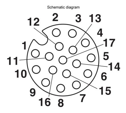
Pin assignment M12, 17-pos., socket side view
