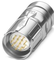
M23, Cable connector, series: CA, straight, shielded: yes, SPEEDCON, No. of pos.: 16, Direction of rotation: Standard, contact connection type: Pin, Solder connection, cable diameter range: 10 mm ... 14.5 mm, coding: N, Alternative product in accordance with RoHS II without Exemption 6c (Pb < 0.1 %) item no.: 1243601
