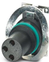
Contact carrier, 3-position, Socket, straight, M8, coding: A, PCB mounting, SMD reflow, Alternative product in accordance with RoHS II without Exemption 6c (Pb < 0.1 %) item no.: 1308261
