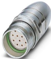
M23, Coupler connector, series: RC, straight, shielded: yes, Screw locking mechanism, No. of pos.: 12, Direction of rotation: Standard, contact connection type: Socket, Solder cup, cable diameter range: 7.5 mm ... 9.5 mm, coding: N, Alternative product in accordance with RoHS II without Exemption 6c (Pb < 0.1 %) item no.: 1241004
