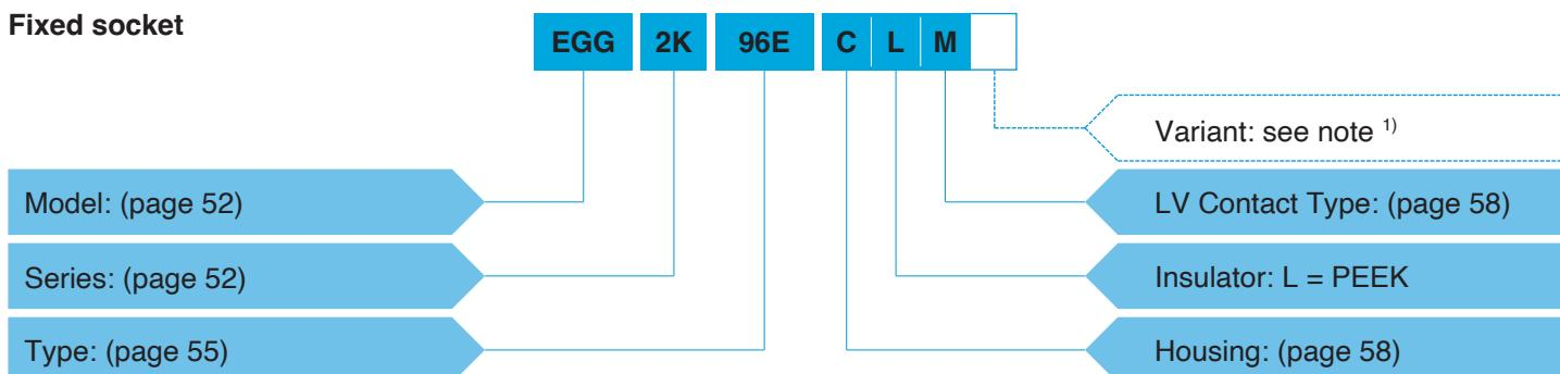
**EGG.2K.96E.CLM** = Fixed socket with key (G), 2K series, hybrid type to accept 1 F1 type fibre optic contact and 6 low voltage contacts, chrome-plated brass housing, PEEK insulator, 6 female crimp electrical contacts.
