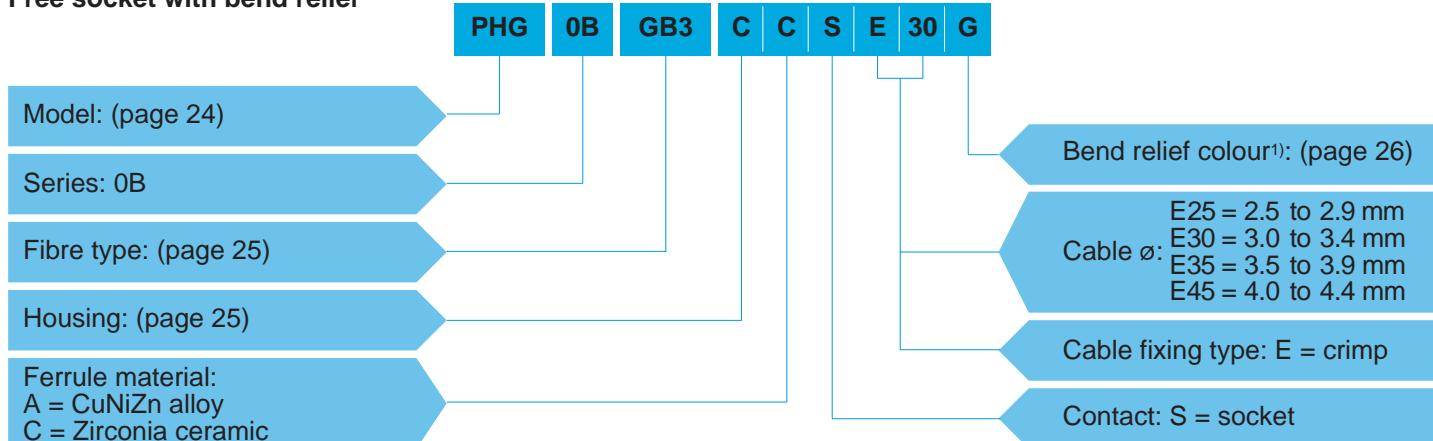
**PHG.0B.GB3.CCS30G** = Free socket with key (G), 0B series, F3 fibre optic contact, ferrule hole diameter 235 µm, chrome-plated brass housing, zirconia ceramic ferrule, socket type contact, crimp type cable fixing for 3.0 to 3.4 mm diameter cable, and gray bend relief.
