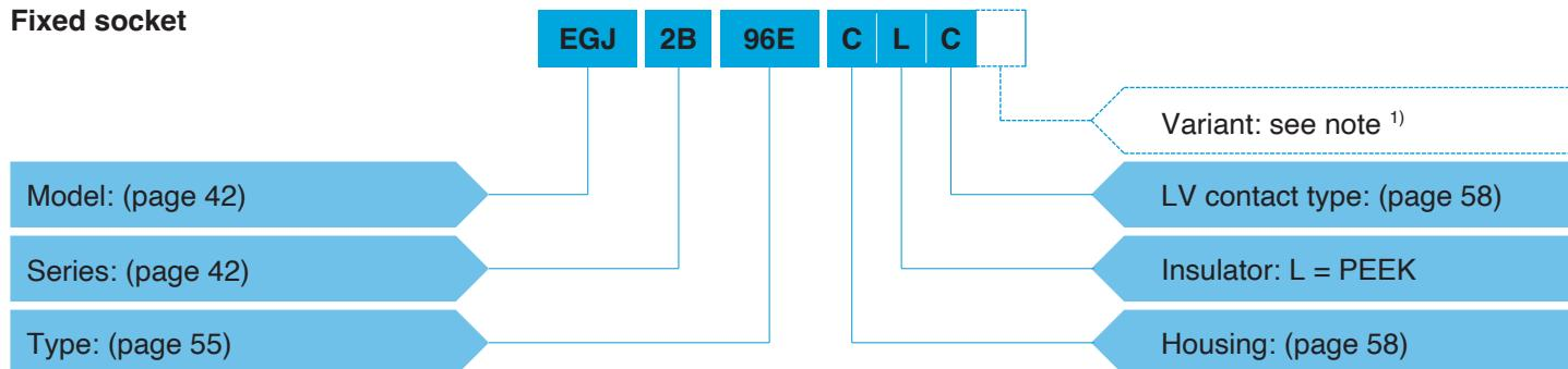
**EGJ.2B.96E.CLC** = Fixed socket with key (code J) 2B series, hybrid type to accept 1 F1 fibre optic contact and 6 low voltage electrical contacts, chrome-plated brass housing, PEEK insulator, 6 male crimp electrical contacts.
