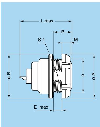
**EEG Fixed socket, nut fixing, key (G) or keys (A...F, L and R) (back panel mounting)**
