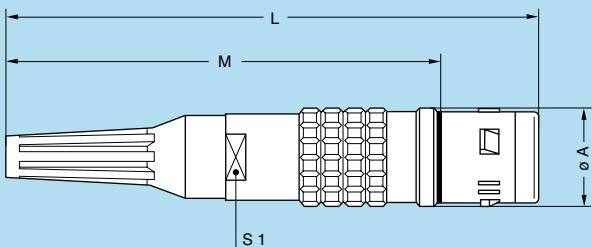
**FGW.3K** Straight plug, keys (W), cable adapter, with bend relief
