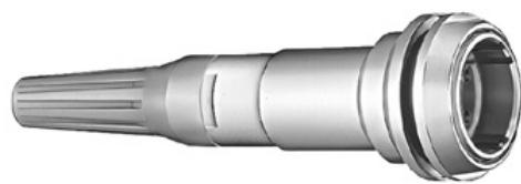
**PEW.3K** Fixed socket, nut fixing, keys (W), cable adapter, with bend relief (back panel mounting)
