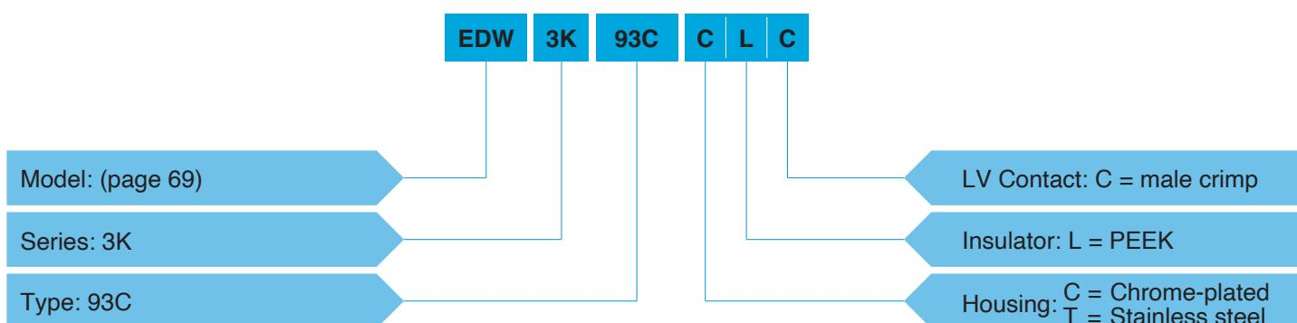
**EDW.3K.93C.CLC** = Fixed socket with rear square flange, keys (W), 3K series, hybrid type to accept 2 F2 type fibre optic contacts, 2 power and 2 signal electrical contacts, chrome-plated brass housing, PEEK insulator, male crimp signal contacts.
