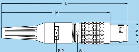
**FGG** Straight plug, key (G) or keys (A...L) cable collet and nut for fitting a bend relief
