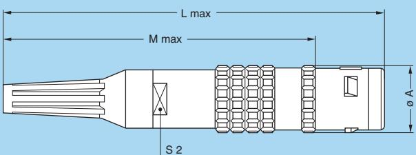
**FGG** Straight plug, key (G) or keys (A...F, L and R), cable adapter and nut for fitting a bend relief
