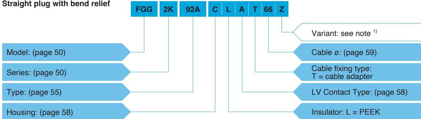
**FGG.2K.92A.CLAT66Z** = Straight plug with key (G), 2K series, hybrid type to accept 1 F2 type fibre optic contact and 2 low voltage contacts, chrome-plated brass housing, PEEK insulator, 2 male solder electrical contacts, cable fixing type T for 6.5 mm diameter cable, and nut for fitting a bend relief.
