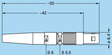
**PKG.00** Fixed socket, nut fixing, key (G) or key (B), with bend relief
