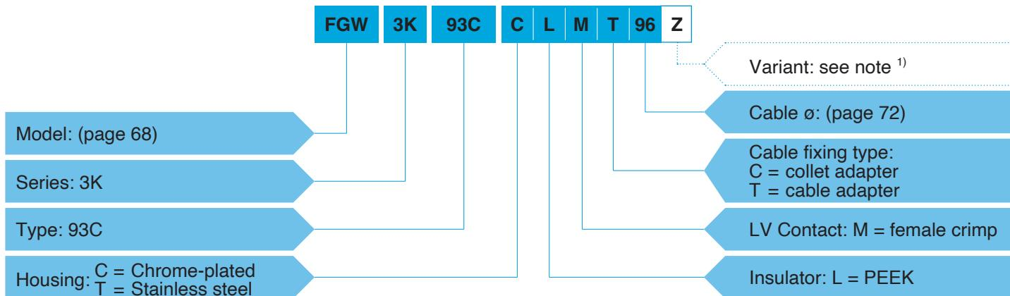
**FGW.3K.93C.CLMT96Z** = Straight plug with keys (W), 3K series, hybrid type to accept 2 F2 type fibre optic contacts, 2 power and 2 signal electrical contacts, chrome-plated brass housing, PEEK insulator, female crimp signal contacts, cable fixing type T for 9.2 mm diameter cable, and nut for fitting a bend relief.
