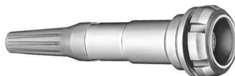
**PEG** Fixed socket, nut fixing, key (G) or keys (A...F, L and R), cable adapter and nut for fitting a bend relief (back panel mounting)
