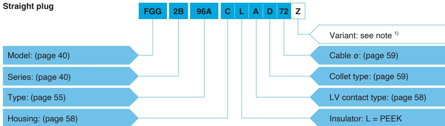
**FGG.2B.96A.CLAD72Z** = Straight plug with key (G), 2B series, hybrid type to accept 1 F1 fibre optic contact and 2 low voltage electrical contacts, chrome-plated brass housing, PEEK insulator, 2 male solder electrical contacts, type D collet system to suit a 7.2 mm diameter cable, and a nut for fitting a bend relief.
