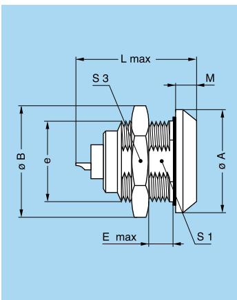
**EGG Fixed socket, nut fixing, key (G) or keys (A...F, L and R)**
