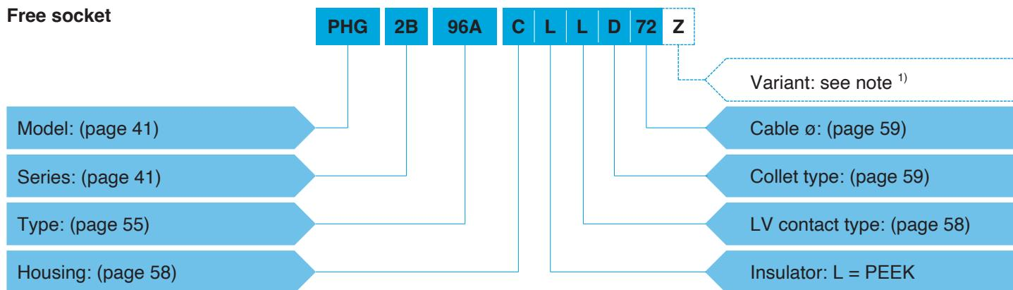
**PHG.2B.96A.CLLD72Z** = Free socket with key (G), 2B series, hybrid type to accept 1 F1 fibre optic contact and 2 low voltage electrical contacts, chrome-plated brass housing, PEEK insulator, 2 female solder electrical contacts, type D collet system to suit a 7.2 mm diameter cable, and a nut for fitting a bend relief.
