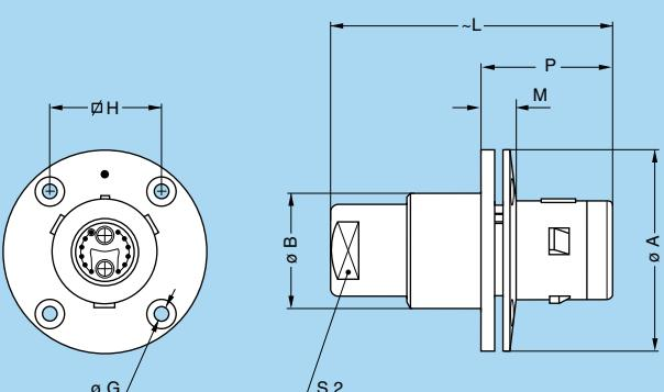
**FXG** Fixed plug with round flange, four holes fixing, key (G) or keys (A...F, L and R)
