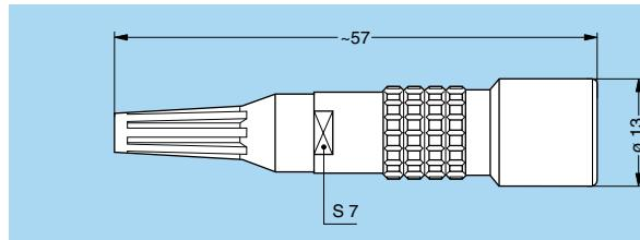
**PEG.0K** Fixed socket, nut fixing, key (G) or keys (A...F) and cable adapter, with bend relief (back panel mounting)
