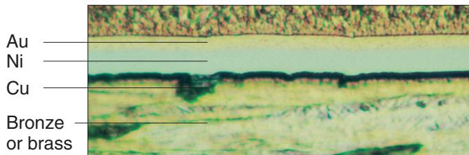
LEMO male solder contacts are made of brass (UNS C 38500). Male crimp contacts are made of brass (UNS C 34500) or annealed brass (UNS C 38500) with optimum hardness (HV) for crimping onto the wire.
