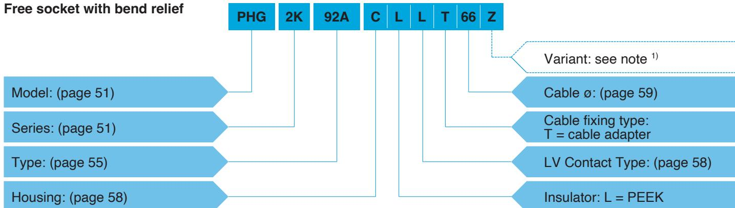
**PHG.2K.92A.CLLT66Z** = Free socket with key (G), 2K series, hybrid type to accept 1 F2 type fibre optic contact and 2 low voltage contacts, chrome-plated brass housing, PEEK insulator, 2 female solder electrical contacts, cable fixing type T for 6.5 mm diameter cable, and nut for fitting a bend relief.
