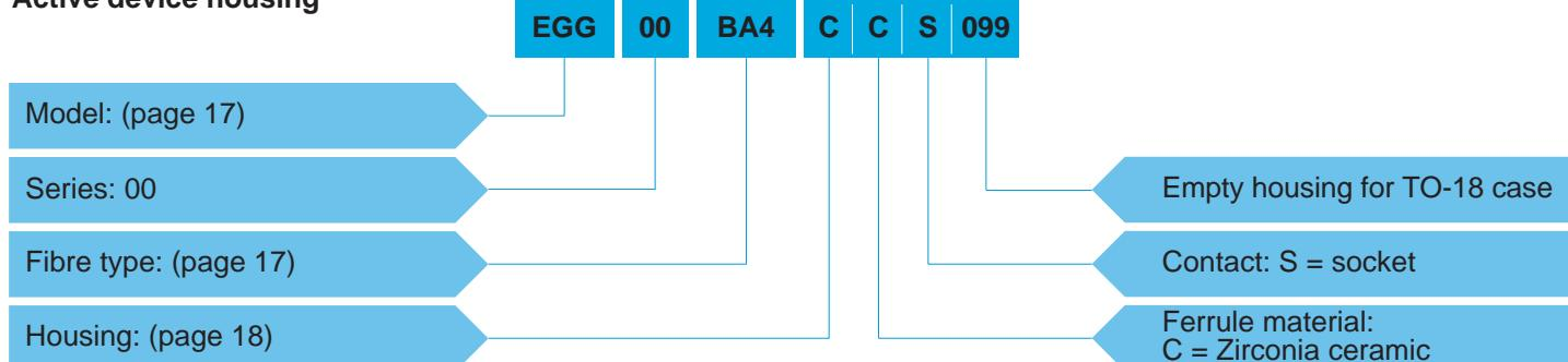
**EGG.00.BA4.CCS099** = Straight active device housing, nut fixing with key (G), 00 series, with ferrule for F4 fibre optic contact, assembled with single-mode fibre ø 9/125, chrome-plated brass housing, zirconia ceramic ferrule, socket contact, empty housing for TO-18 case.
