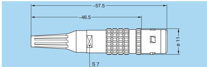
**PKG.0K** Fixed socket, nut fixing, key (G) or keys (A...F) and cable adapter, with bend relief
