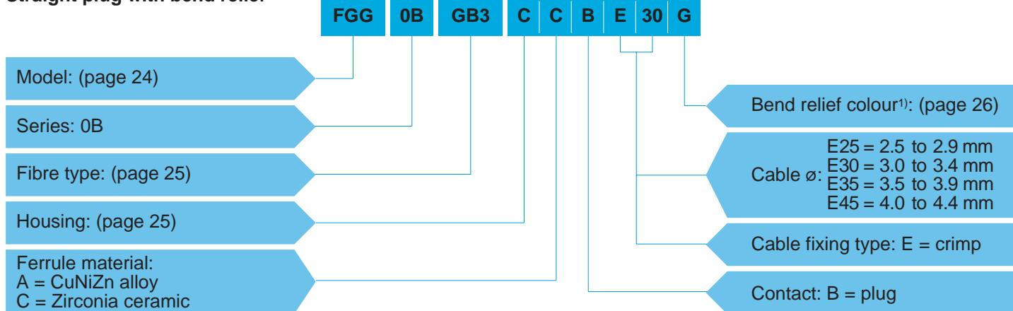
**FGG.0B.GB3.CCB30G** = Straight plug with key (G), 0B series, F3 fibre optic contact, ferrule hole diameter 235 µm, chrome-plated brass housing, zirconia ceramic ferrule, plug type contact, crimp type cable fixing for 3.0 to 3.4 mm diameter cable, and gray bend relief.
