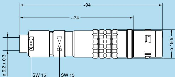
**FUW.3K** Straight plug, keys (W), cable collet adapter and long shell for fitting a bend relief with cap (with enhanced screen efficiency)
