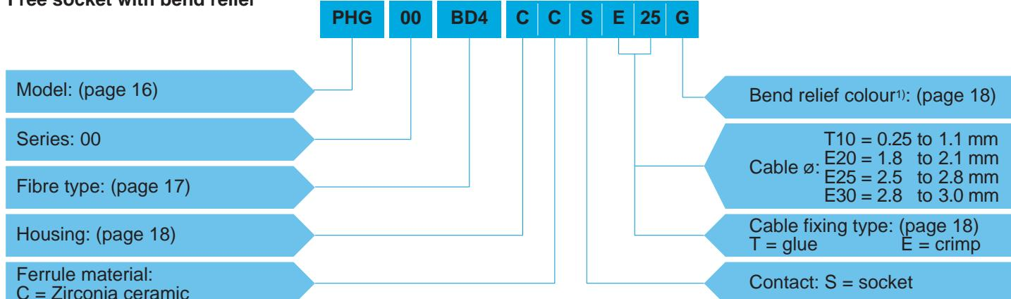
**PHG.00.BD4.CCSE25G** = Free socket with key (G), 00 series for single-mode or multi-mode fibres, F4 fibre optic contact, ferrule hole diameter 128 µm, chrome-plated brass housing, zirconia ceramic ferrule, socket type contact, crimp type cable fixing for 2.5 to 2.8 mm diameter cable, and gray bend relief.
