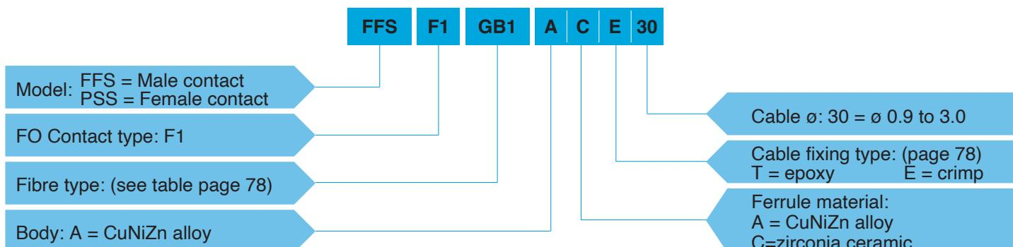
**FFS.F1.GB1.ACE30** = Male F1 type fibre optic contact, ferrule bore diameter of 235  $\mu\text{m}$ , ferrule made of zirconia ceramic, crimp type cable fixing for a cable diameter of 0.9 mm to 3.0 mm.
