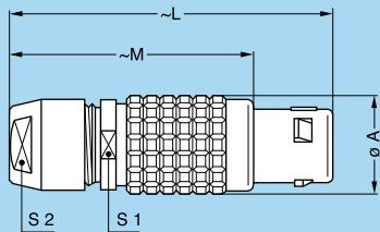
**FGG** Straight plug, key (G) or keys (A...L and R) and cable collet
