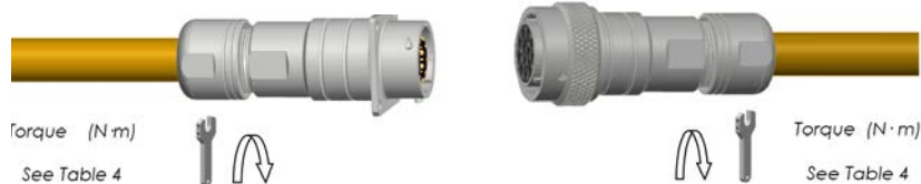
Step 13: Tighten metal nut
