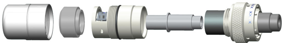
Step 1: Slide components onto cable
