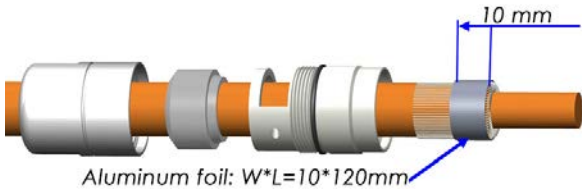
Step 4: Wrap foil over braided shielding
