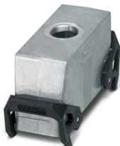
Sleeve housing B24, with double locking latch, material: Die-cast aluminum, salt water resistant, cable outlets: 1, straight, 1x Pg29, height: 60 mm, cable gland: none, Standard
