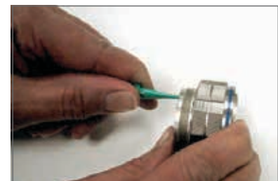
Plastic tool with contact in proper position.
