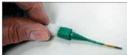
Plastic tool with contact in proper position.
