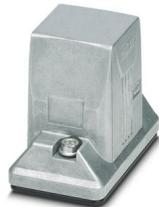
Sleeve housing B6, with screw locking, material: Die-cast aluminum, salt water resistant, variable, height: 74 mm, cable gland: none, Offshore/EMC, Without thread opening for screw connection, conductive seal (EMC properties)
