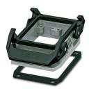
Panel mounting base D50, with double locking latch, material: Die-cast aluminum, salt water resistant, height: 32 mm, cable gland: none, Standard, with flat gasket
