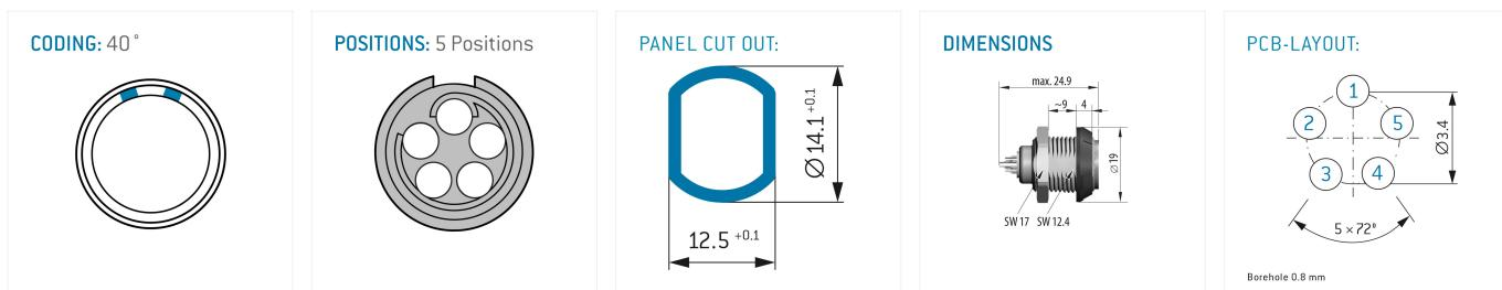
The pin layout corresponds to the view on the termination area
