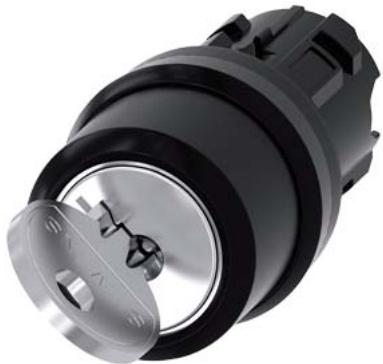
RONIS key-operated switch, 22 mm, round, plastic, lock number 455, with 2 keys, 2 switch positions O-I, latching, actuating angle 90°, 10:30h/13:30h, key removal O, with laser labeling, lower case
