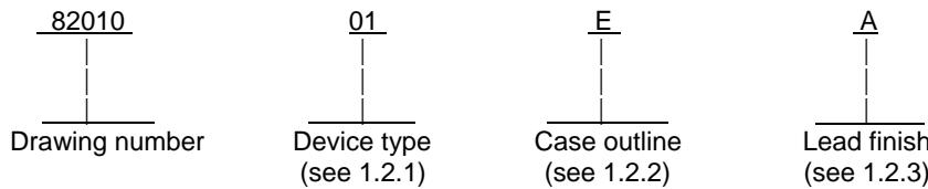
1.2.1 Device types. The device types shall identify the circuit functions as follows:
