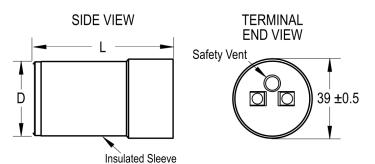
General Information Series MS/A902 Dielectric Aluminum Electrolytic Style Motor Start Description Motor Start Aluminum Electrolytic RoHS Lead **Quick Connect** AEC-Q200 No Halogen Free true Shelf Life 156 Weeks
