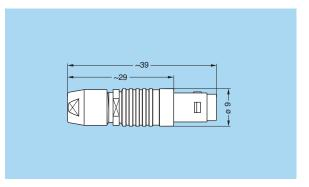
FGG Straight plug, cable collet and nut for fitting a bend relief
