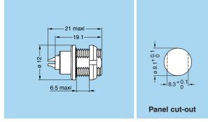
**HGG** Fixed socket, nut fixing, watertight or vacuumtight
