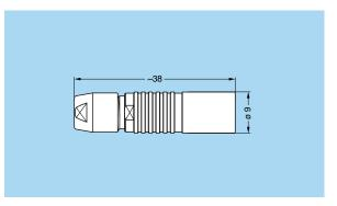
PHG Free socket, cable collet and nut for fitting a bend relief
