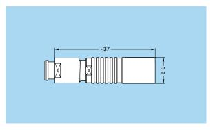
FGG Straight plug, cable collet and nut for fitting a bend relief, POM outer shell
