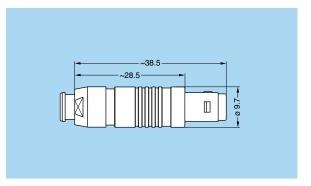
EGG Fixed socket, nut fixing, POM outer shell
