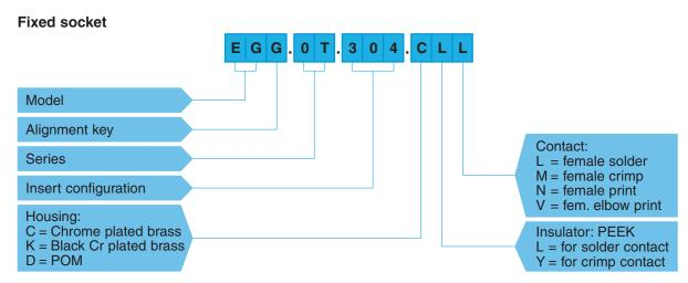
**EGG.0T.304.CLL** = fixed socket, nut fixing, with key (G), 0T series, multipole type with 4 contacts, outer shell in chrome-plated brass, PEEK insulator, female solder contacts.
