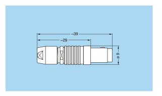
**EGG** Fixed socket, nut fixing
