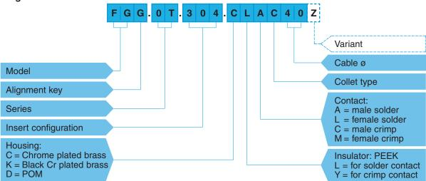
**FGG.0T.304.CLAC40Z** = Straight plug with key (G) and cable collet for bend relief, 0T series, multipole type with 4 contacts, outer shell in chrome-plated brass, PEEK insulator, male solder contacts, C type collet for 4.0 mm diameter cable and nut for fitting a bend relief.
